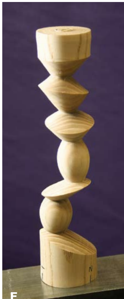
This circular-type spindle includes three twisted axes.
