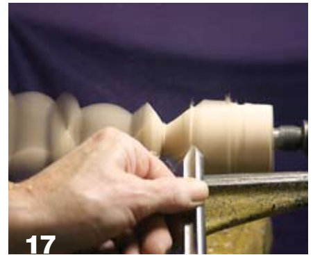
17 On Axis 3, make a V-cut. Because you're contacting air wood, light cuts work best.
