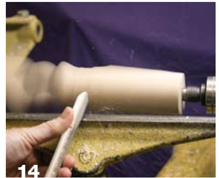
14 When beginning to cut the second bead, take light cuts to avoid catches in air wood.
