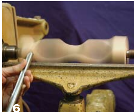
With the lathe turning, the air wood takes on a different profile.
