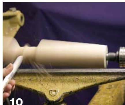
With a spindle gouge, remove all of the air wood and turn a cylinder.
