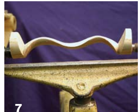
When complete, the turning on Axis 2 reveals a delicate spindle.
