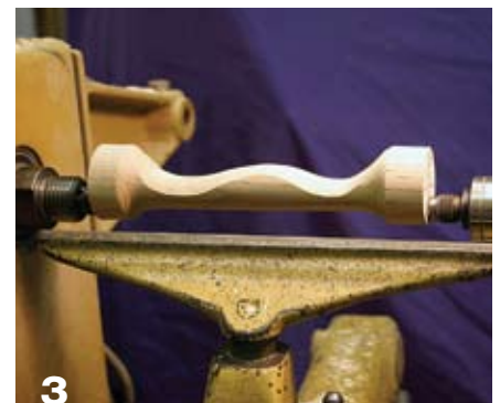
3 On Axis 1, turn two beads and a cove with a spindle gouge.
