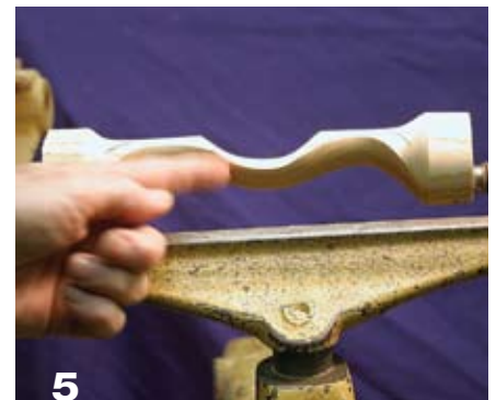
5 With the lathe stopped, the Axis 2 changes are evident on the spindle.
