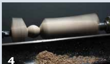
4 A new axis, positioned close to the center axis, allows enough solid wood for a circular outcome, in this case, a bead.
