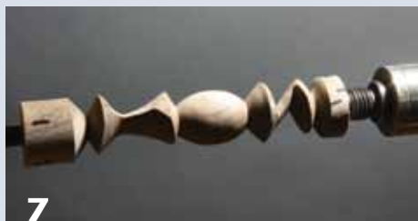
7 From the starting point of a bead turned on the central axis (see Photo 6), additional profiles are turned using other axes.
