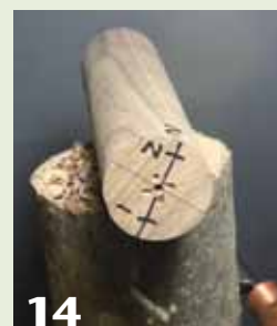
14 Write the axes numbers on the ends and sides of the cylinder so they are clearly visible. Even with a numbering system, though, mistakes are easy to make.
