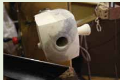
An exploration in multiaxis turning can combine spindle turning with faceplate turning.
