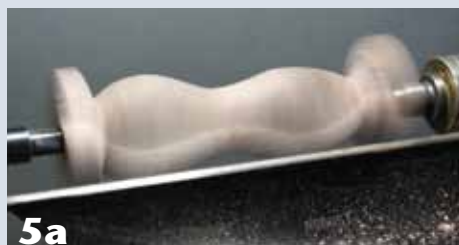
5a A new axis, located close to the outside of the spindle, results in substantial air-wood. An arc-type outcome is possible.
