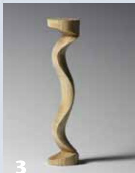
3 This arc-type multiaxis spindle has two axes parallel to the center axis and they are in the same plane.
